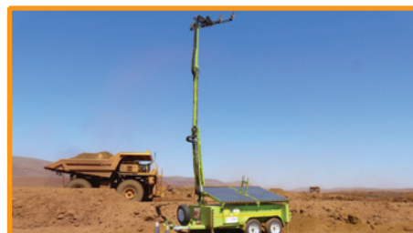
SOLAR LIGHTING TOWER
